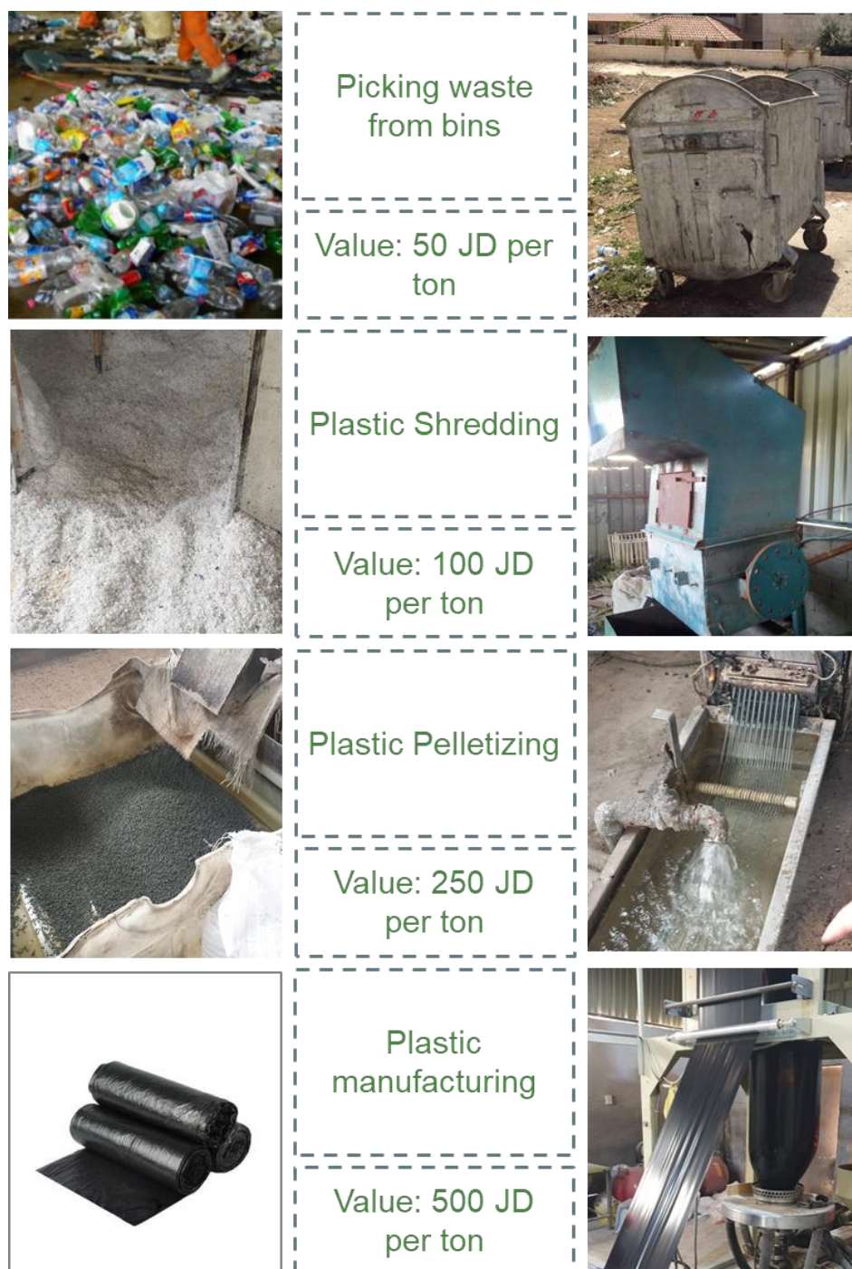
Figure 10 Example of Common Plastic Recycling Cycle for PE in Jordan
