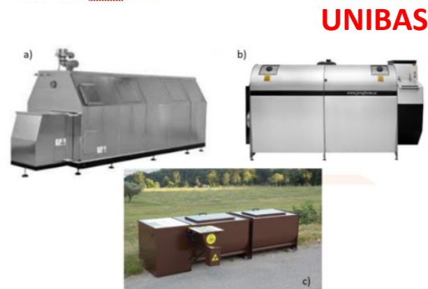
Figure 5. Example of community composters: a) rotating chamber system; b) and c) two chamber systems
